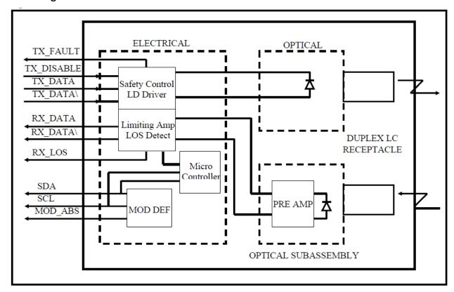
**Transmitter Section-** The FP laser driver accept differential input data and provide bias and modulation currents for driving a laser. An automatic power-control (APC) feedback loop is incorporated to maintain a constant average optical power. 1550nm FP in an eye safe optical subassembly (OSA) mates to the fiber cable.
